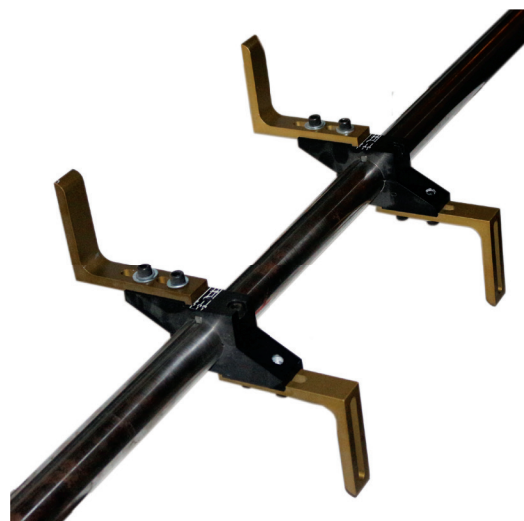
Figure 2 Picture showing one finger set on one axis of a typical machine. Fingers are adjustable along the axis. The servomotor that drives this axis is not shown.
