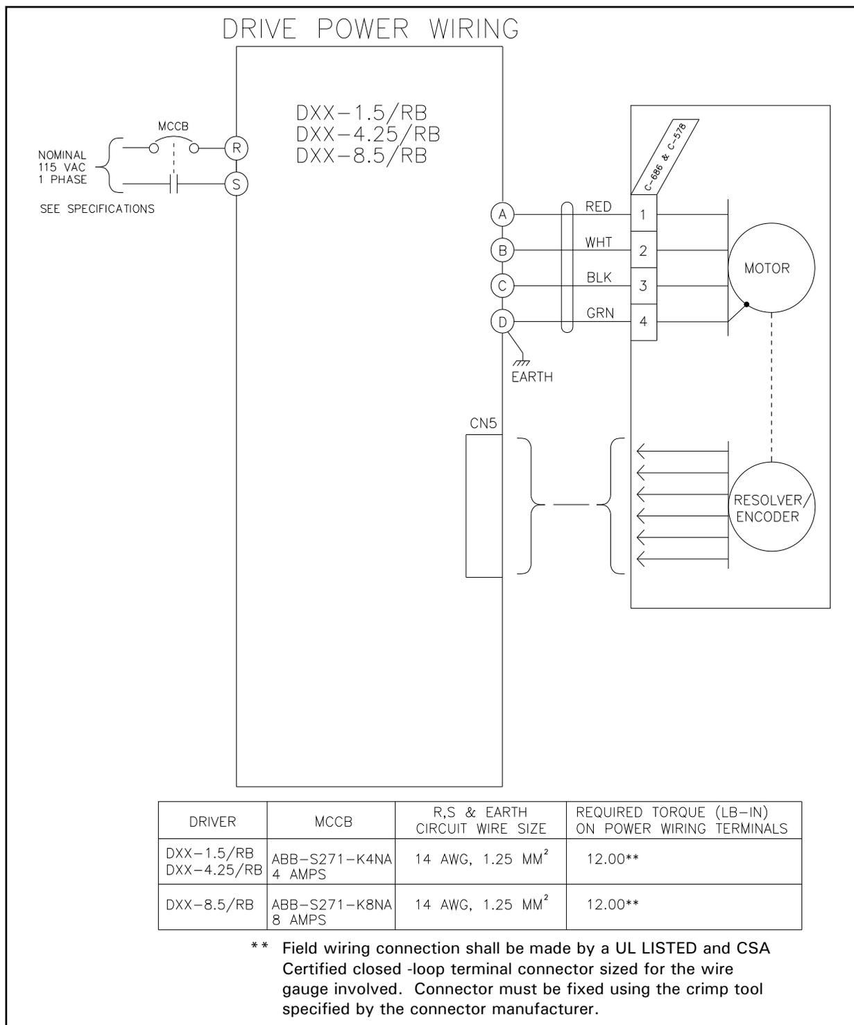
**Figure 6.3 - DS-1.5/RA Through DS-17.5/RA Power Wiring**
