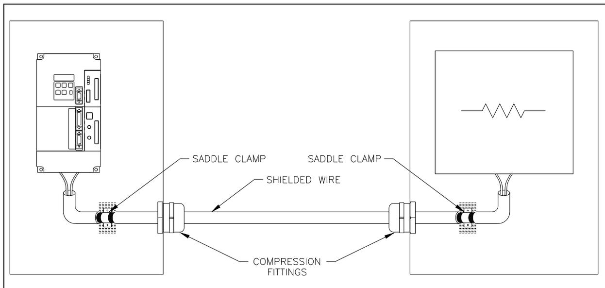
**Figure 13.9 - Saddle Clamp Method of Grounding**
