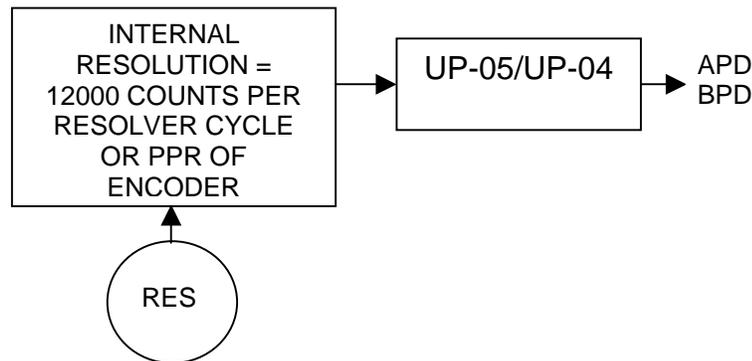
**Example:** It is desired to output 8192 pulses/revolution of the motor shaft. A motor with a 2x resolver would have an internal resolution of  $2 \times 12000 = 24000$  counts/rev of the motor. The internal driver resolution must be multiplied by  $8192/24000$ . Set UP-04 to 24000 and UP-05 to 8192. Any ratio equivalent to  $8192/24000$  will also work like  $4096/12000$ ,  $128/375$ , etc.
