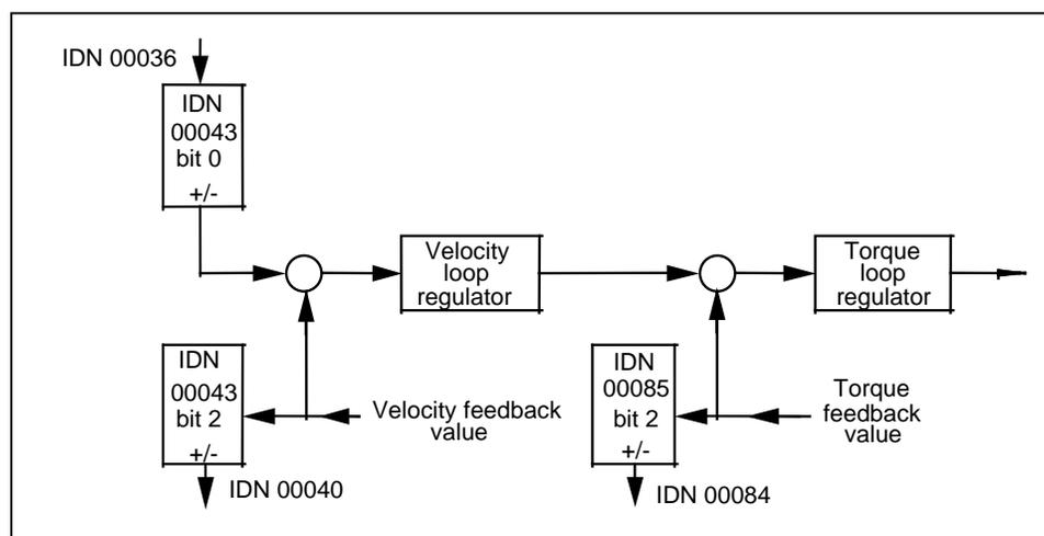
Figure 5.1 - Velocity Polarity Parameter
