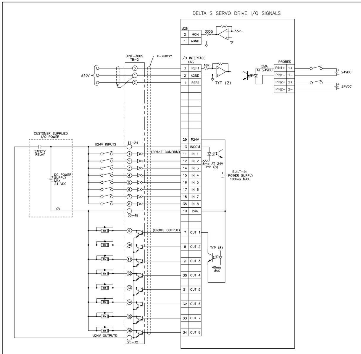
Figure 7.2 - I/O Connections To a DINT-300S
