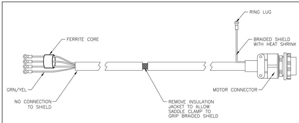
Figure 13.7 - Alternate Method to Ground the Motor Armature Cable
