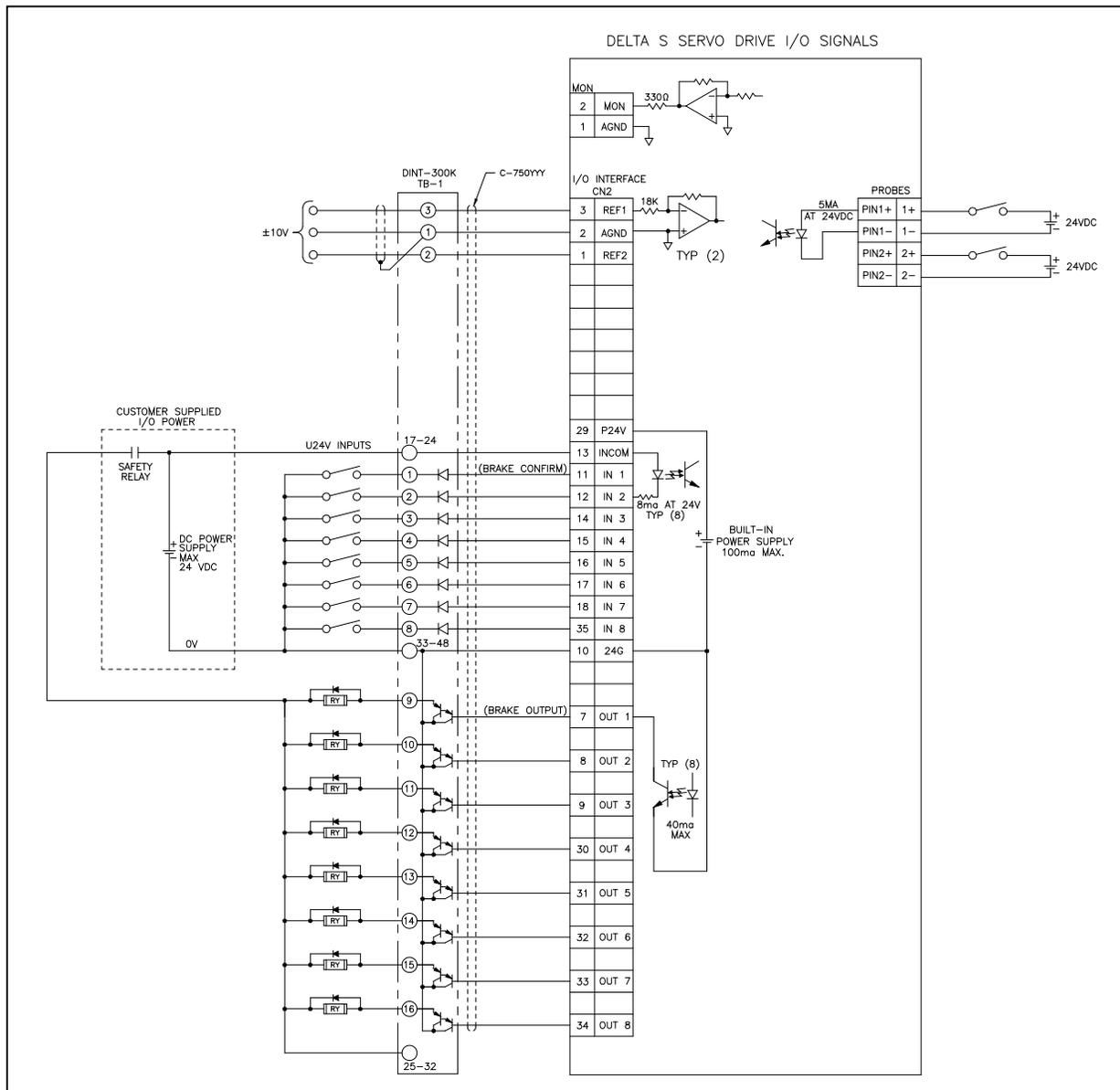
Figure 7.3 - I/O Connections To a DINT-300K
