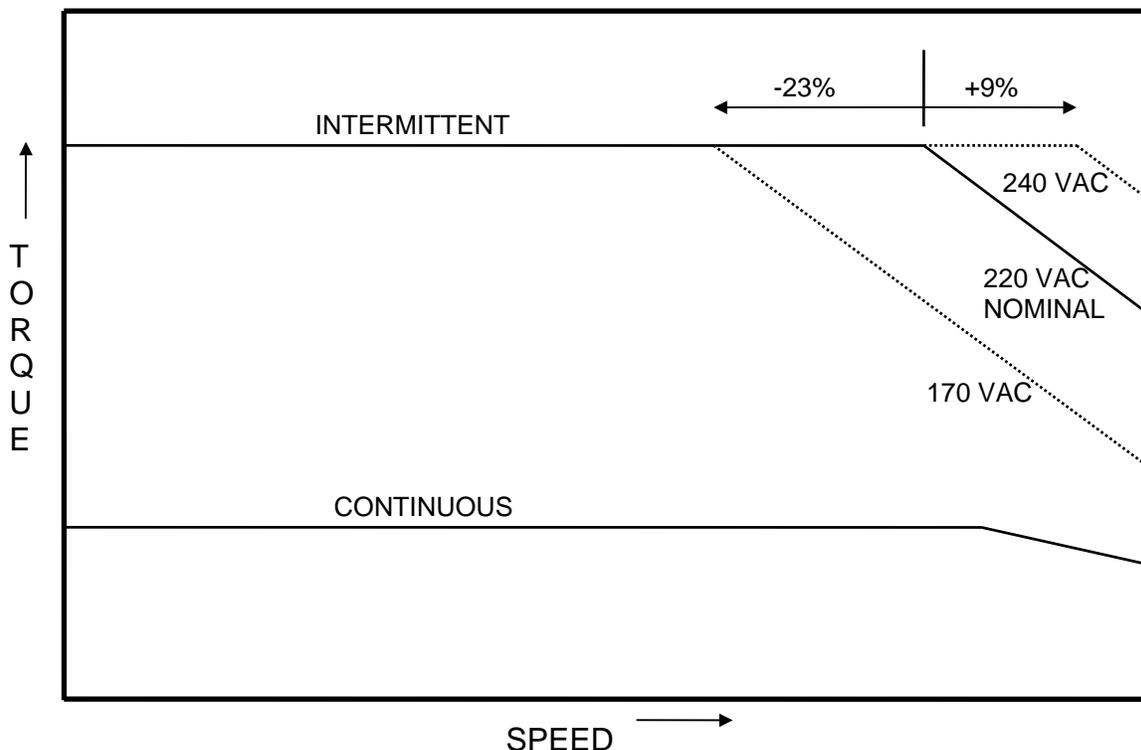
As the servo motor speed goes up, the counter EMF or generator action of the motor increases the voltage across the motor windings. The driver must provide a voltage greater than the motor voltage to produce current in the winding and therefore torque at the motor shaft. The intermittent torque curve rolls off when the motor voltage reaches the driver's internal DC bus voltage. The internal DC bus voltage is directly related to the incoming line voltage.
