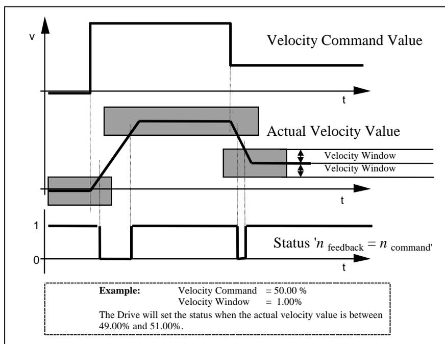
Figure 5.4 - Example of Velocity Window
