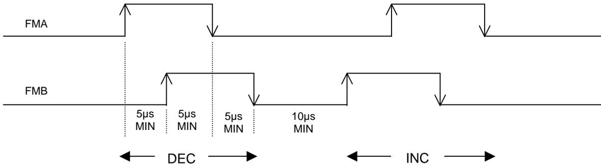
**PULSE AND DIRECTION DECODING (UP-18 = 02)** where FMA is pulse count and FMB is direction. Maximum frequency of FMA is 200 KHZ.
