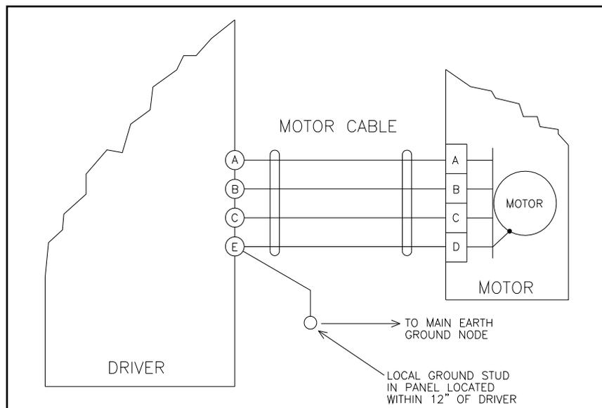
Figure 6.1 - Grounding Technique
