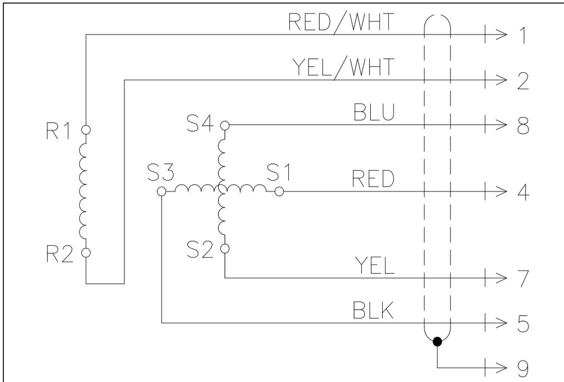
**Figure 3.6 - Standard Resolver Wiring Connections for
