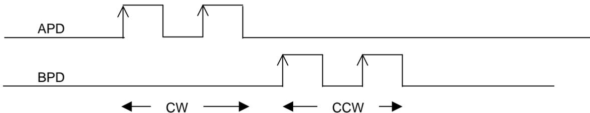
**AB QUADRATURE DECODING (UP-19 = 01)** where APD leads BPD for CCW motor rotation. Maximum frequency of APD and BPD is 100 KHZ. This mode simulates an encoder output being read as 4X.
