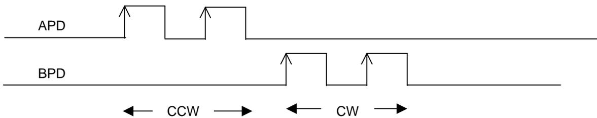
**PULSE-PULSE DECODING (UP-19 = 10)** where APD pulses when the motor actual position moves CW and BDP pulses when the motor actual position moves CCW. Maximum frequency of FMA and FMB is 400 KHZ.
