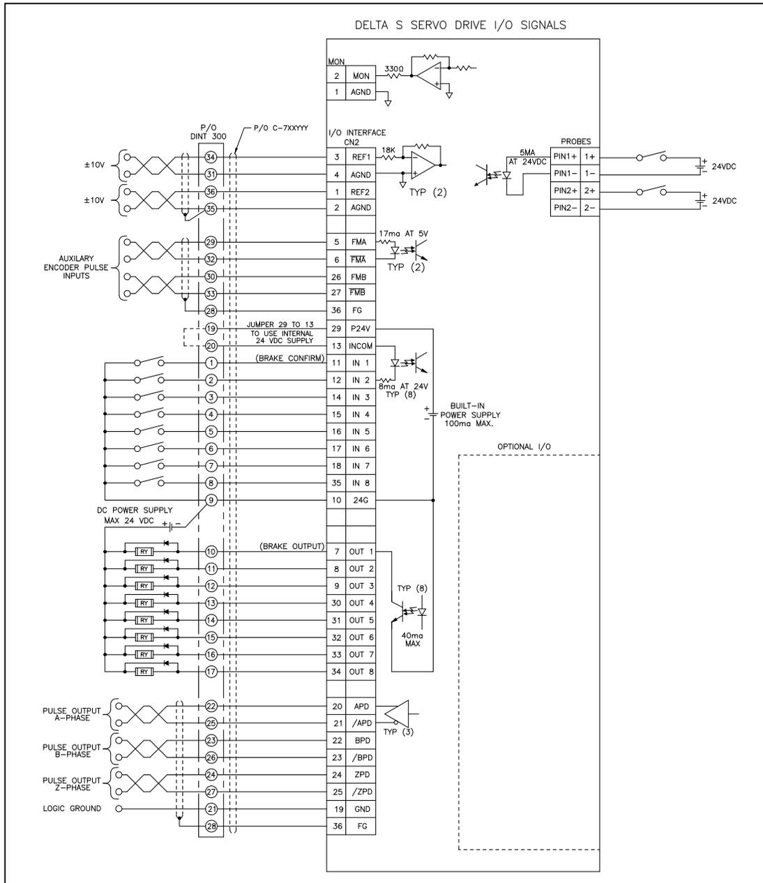
Figure 7.1 - I/O Connections To a DINT-300
