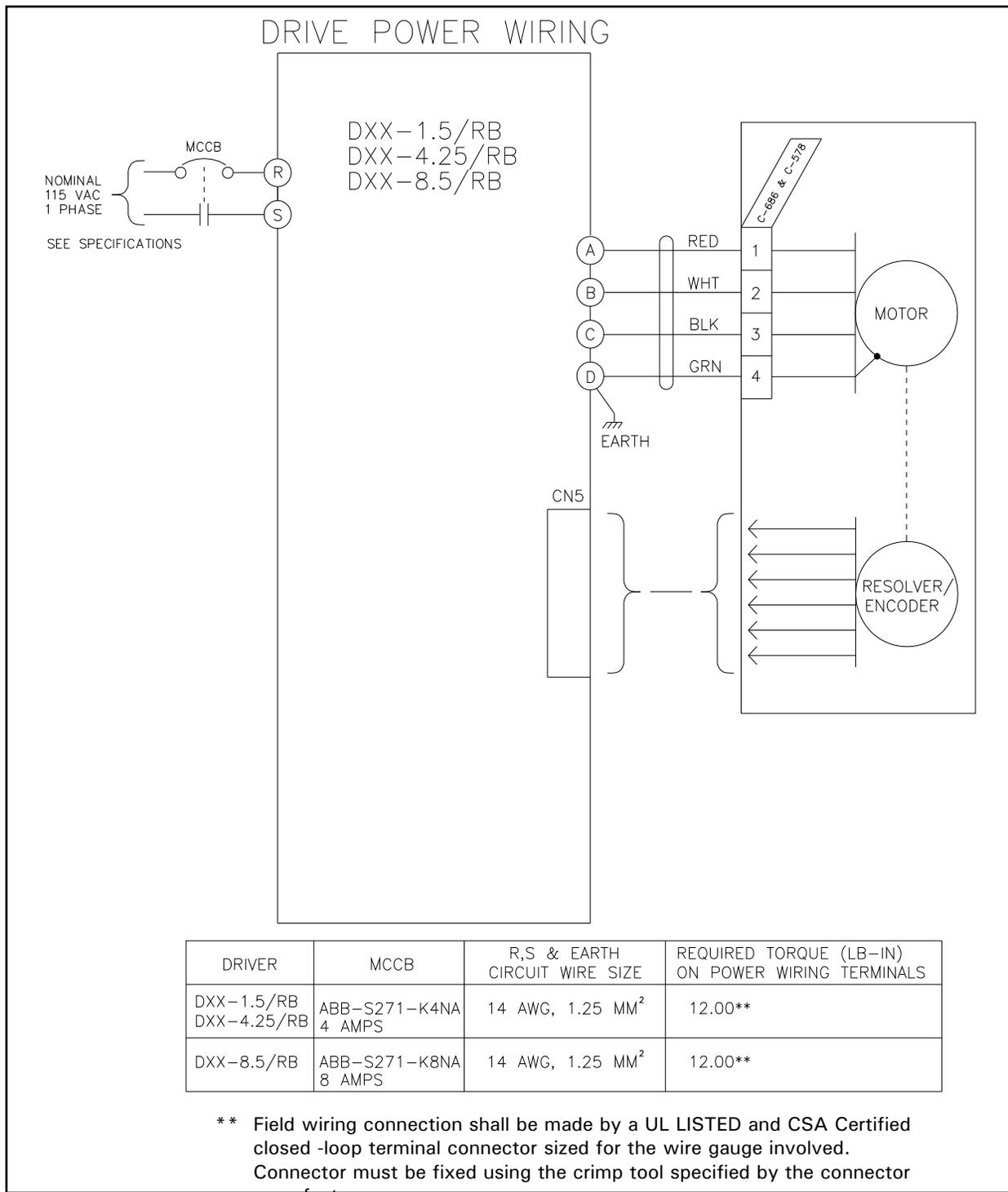
**Figure 6.2 - DS-1.5/RB Through DS-8.5/RB Power Wiring**
