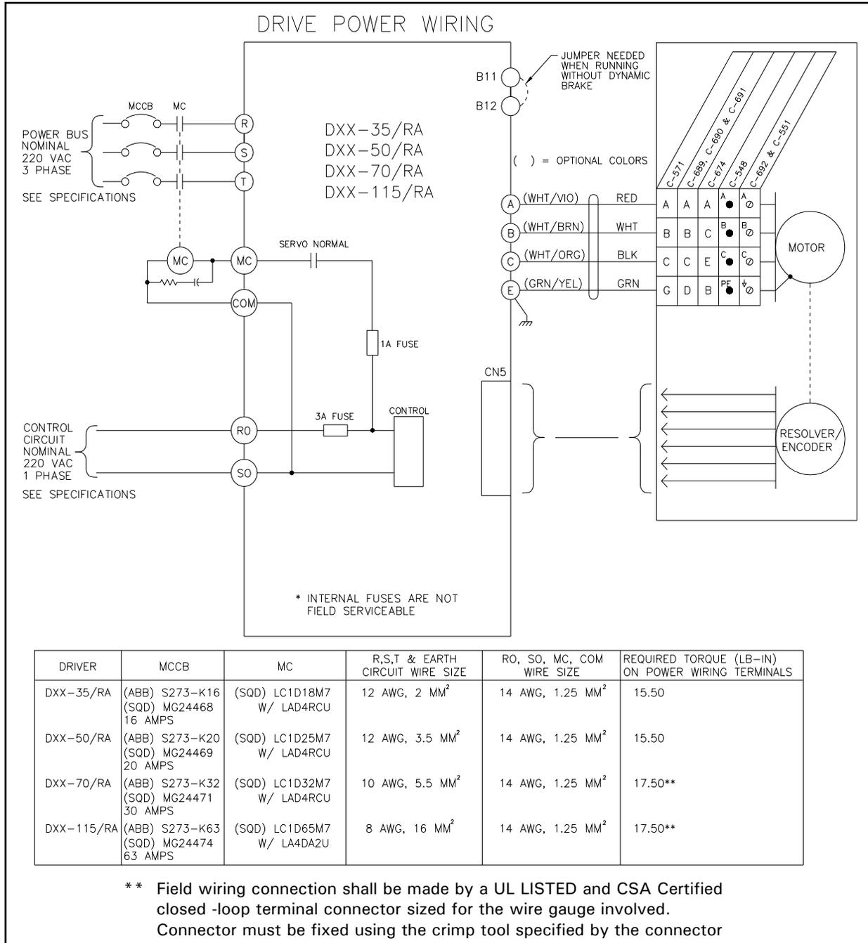
**Figure 6.4 - DS-35/RA Through DS-115/RA Power Wiring**
