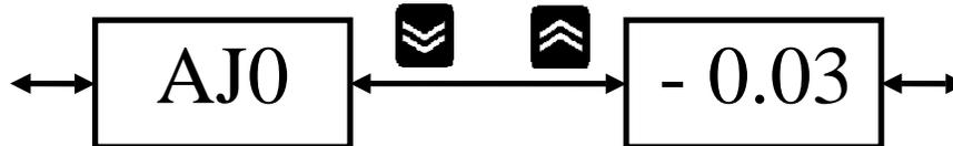
Parameters can be read or written in the Adjust Parameter Menu Loop. The procedure to write into a parameter is found in **Section 4.2**.
