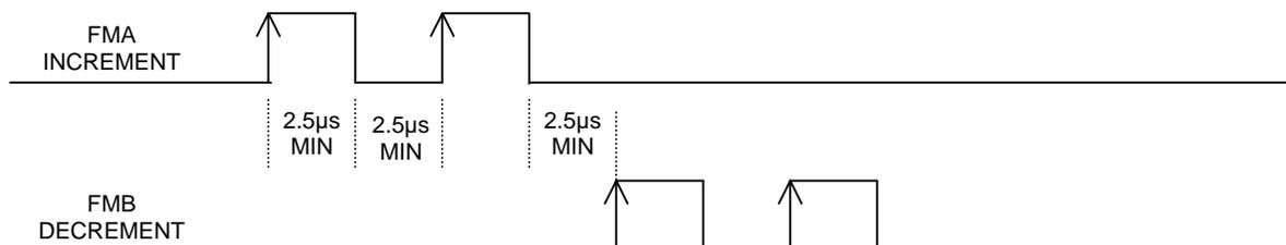
**PULSE-PULSE DECODING (UP-18 = 10)** where FMA decrements the command position and FMB increments the encoder position. Maximum frequency of FMA and FMB is 200 KHZ.
