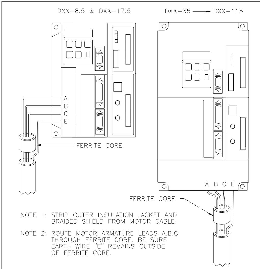
**Figure 13.3 - Driver Output (Motor Armature) Filter**
