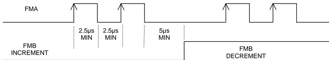
**PULSE AND DIRECTION DECODING (UP-18 = 12)** where FMA is pulse count and FMB is direction. Maximum frequency of FMA is 200 KHZ.
