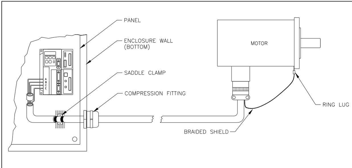
Figure 13.6 - Alternate Method to Ground the Motor Armature Cable
