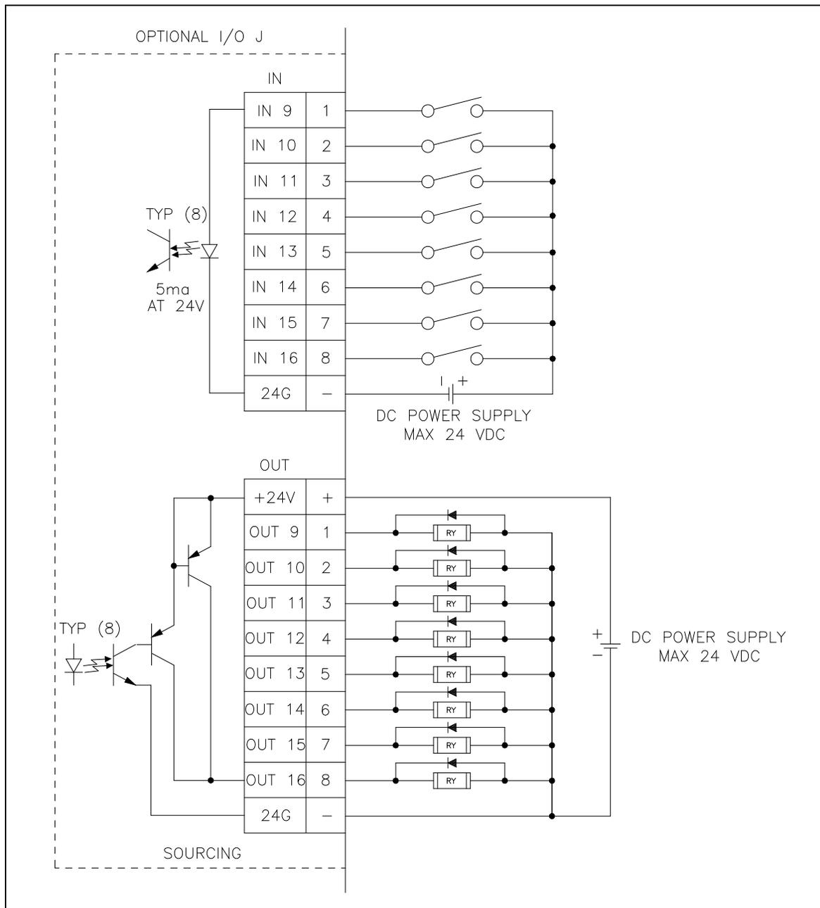
Figure 7.4 - I/O Connections For Optional J (Sourcing) Board
