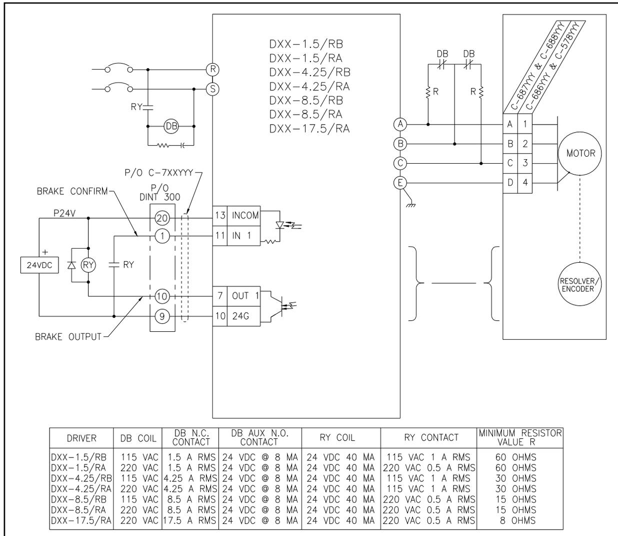
Figure 10.1 - Dynamic Brake Connection for the DS-1.5 Through DS-17.5 Drivers
