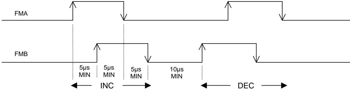
**AB QUADRATURE DECODING (UP-18 = 11)** where FMB leading FMA increments the command position, FMA leading FMB decrements the encoder position. Maximum frequency of FMA and FMB is 50 KHZ.
