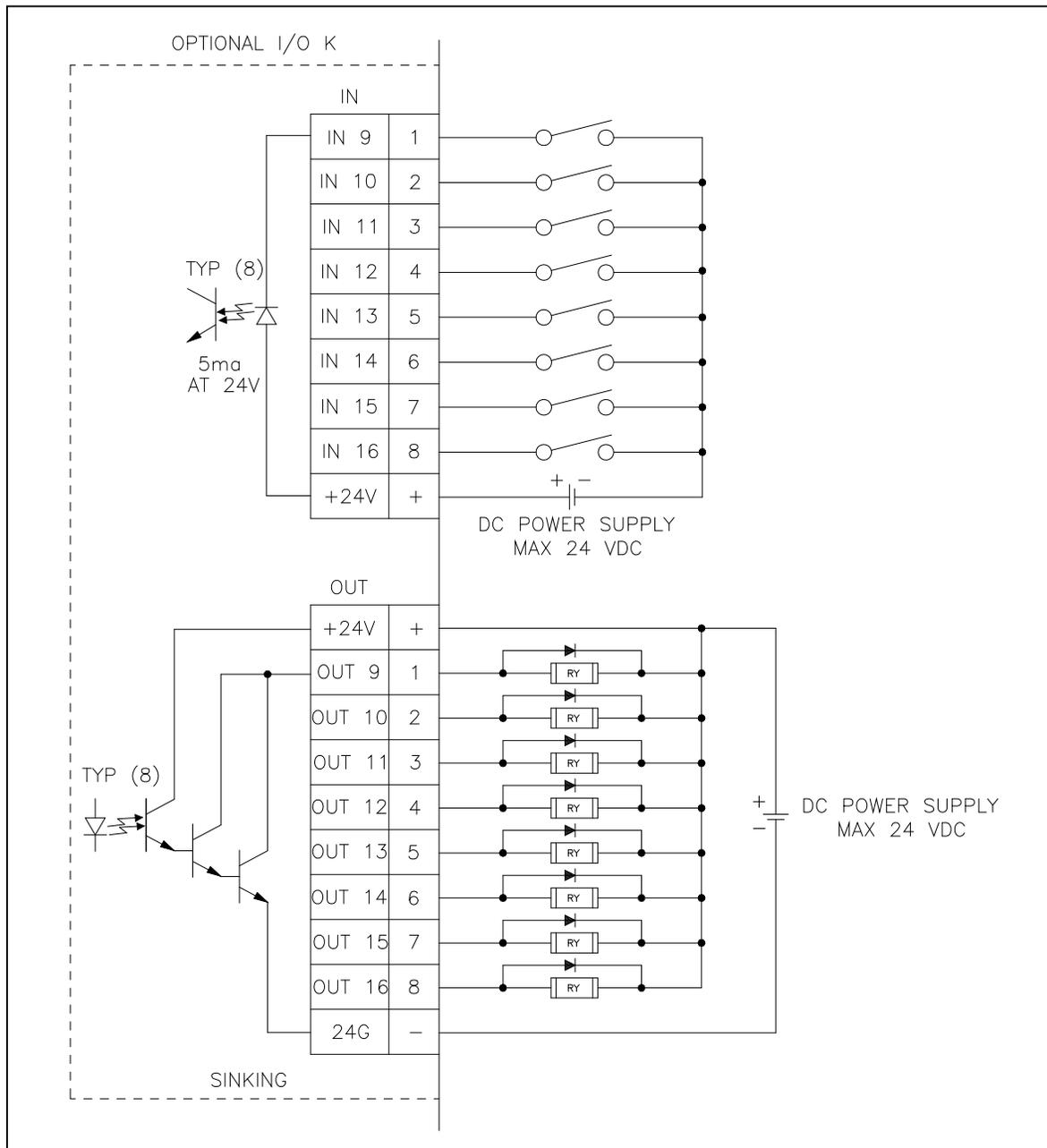
Figure 7.5 - I/O Connections For Optional K (Sinking) Board
