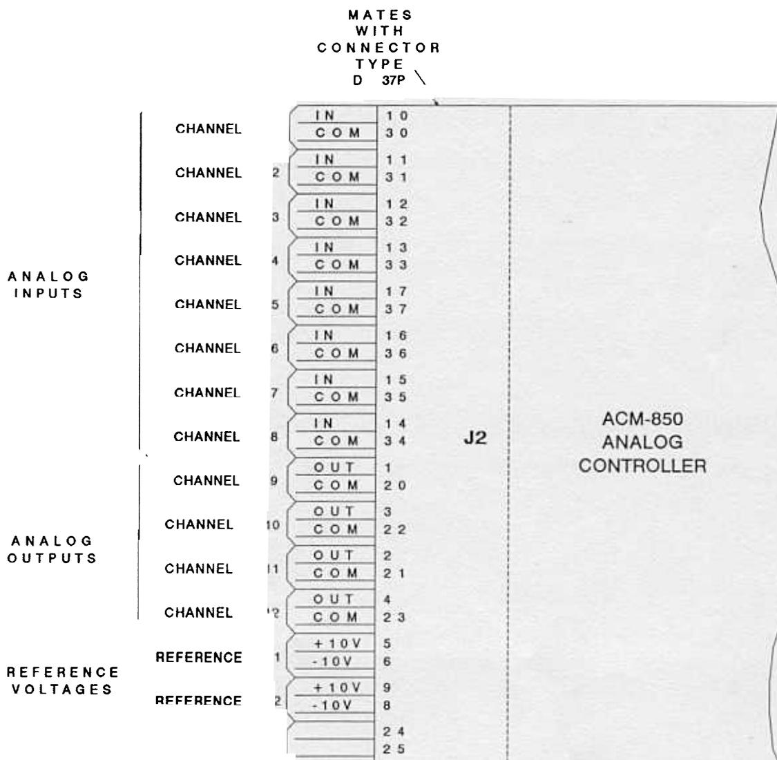
Figure 6-1 ACM-850 Controller, Electrical Connections
