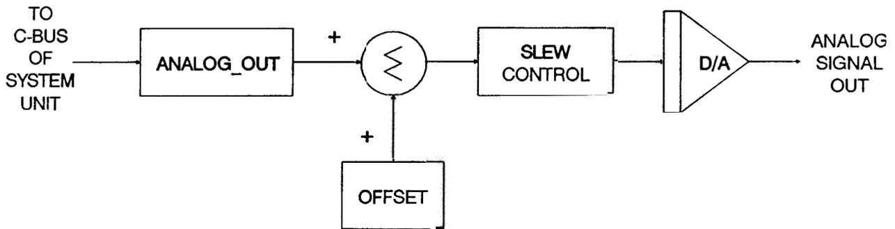
Figure 2-4 Analog Output Channel, Block Diagram
