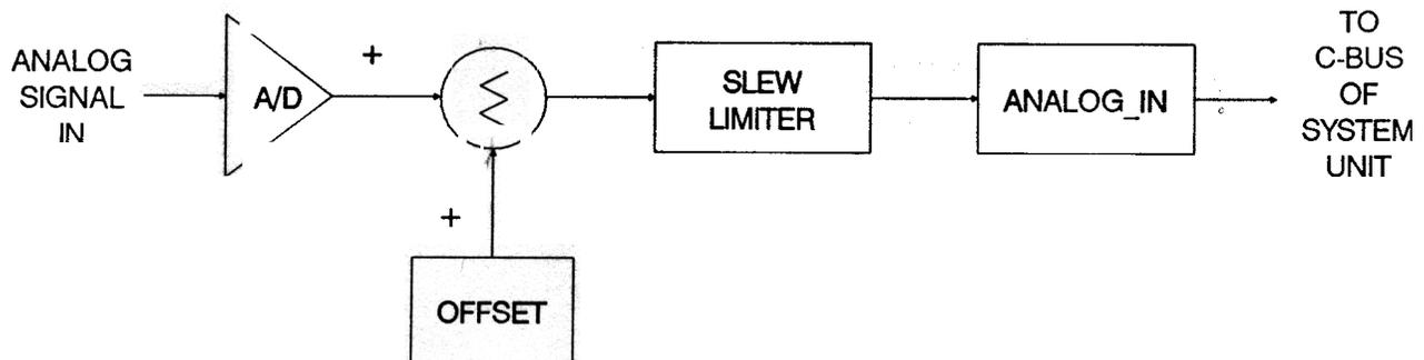
Figure 2-1 Analog Input Channel, Block Diagram
