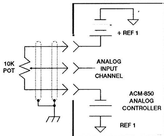
Figure 2-6 Reference Voltage Interface to a Potentiometer
