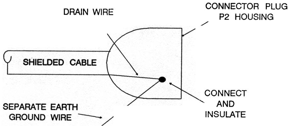
Figure 6-2 Recommended Cable Shielding Connection Technique
