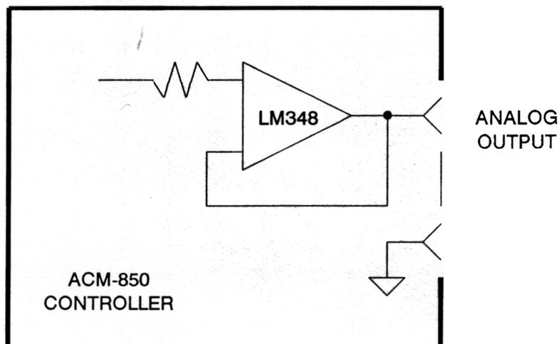
Figure 2-5 Analog Output Circuit
