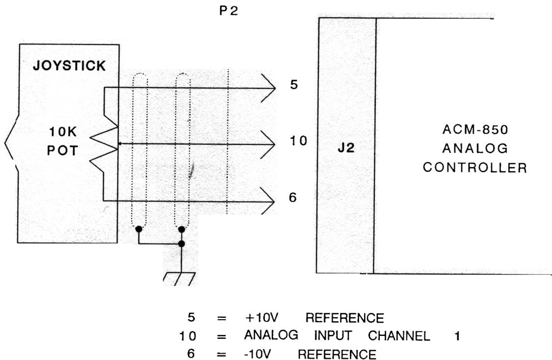
Figure 6-3 Typical Potentiometer User Connection
