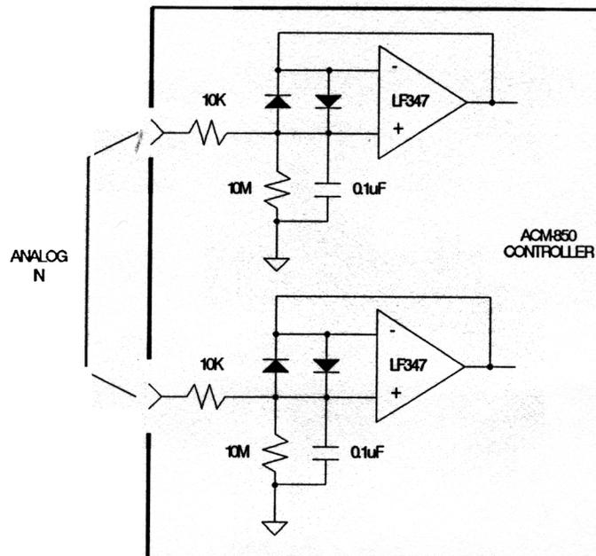
Figure 2-3 Balanced Analog Input Circuits
