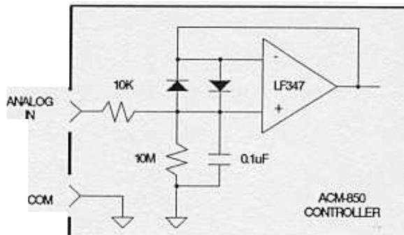
Figure 2-2 Unbalanced Analog Input Circuit
