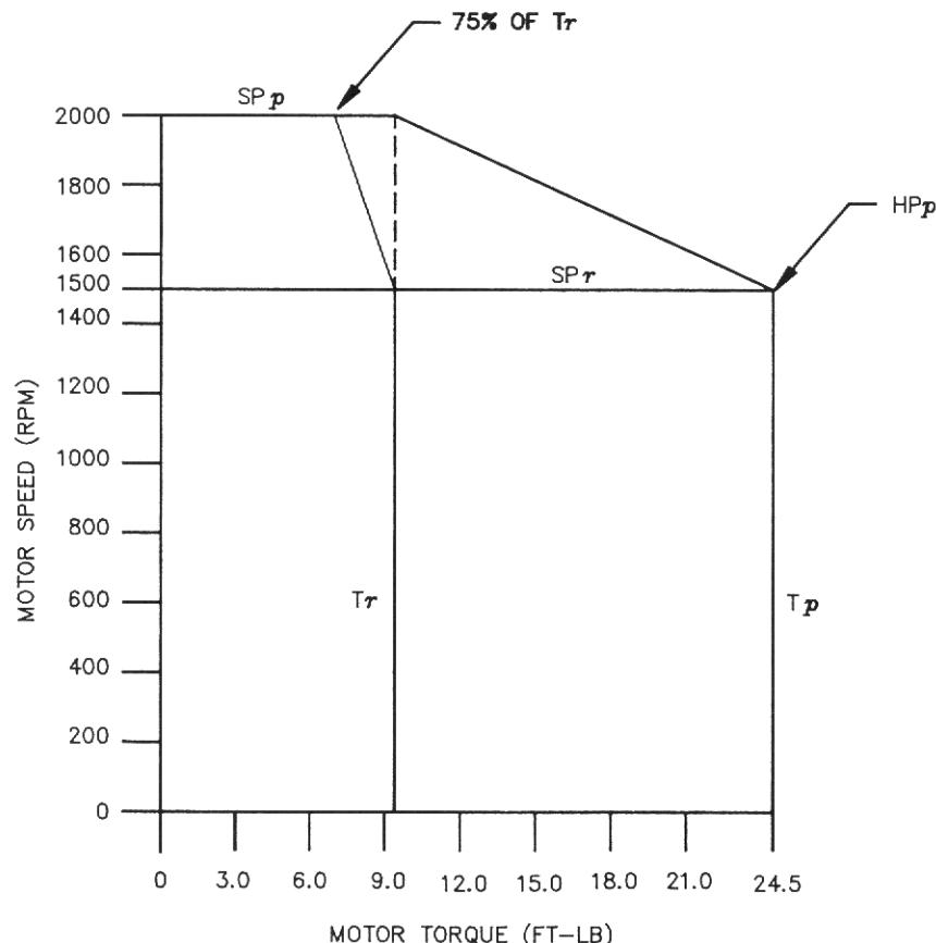
SPEED TEST POINT SCALING: SPEED (RPM) = OUTPUT VOLTS \* SSCL (PARAMETER SSCL DEFAULTS TO 2000 RPM)
