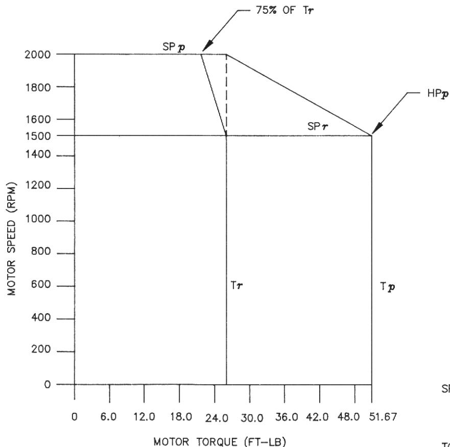
SPEED TEST POINT SCALING: SPEED (RPM) = OUTPUT VOLTS \* SSCL ( PARAMETER SSCL
