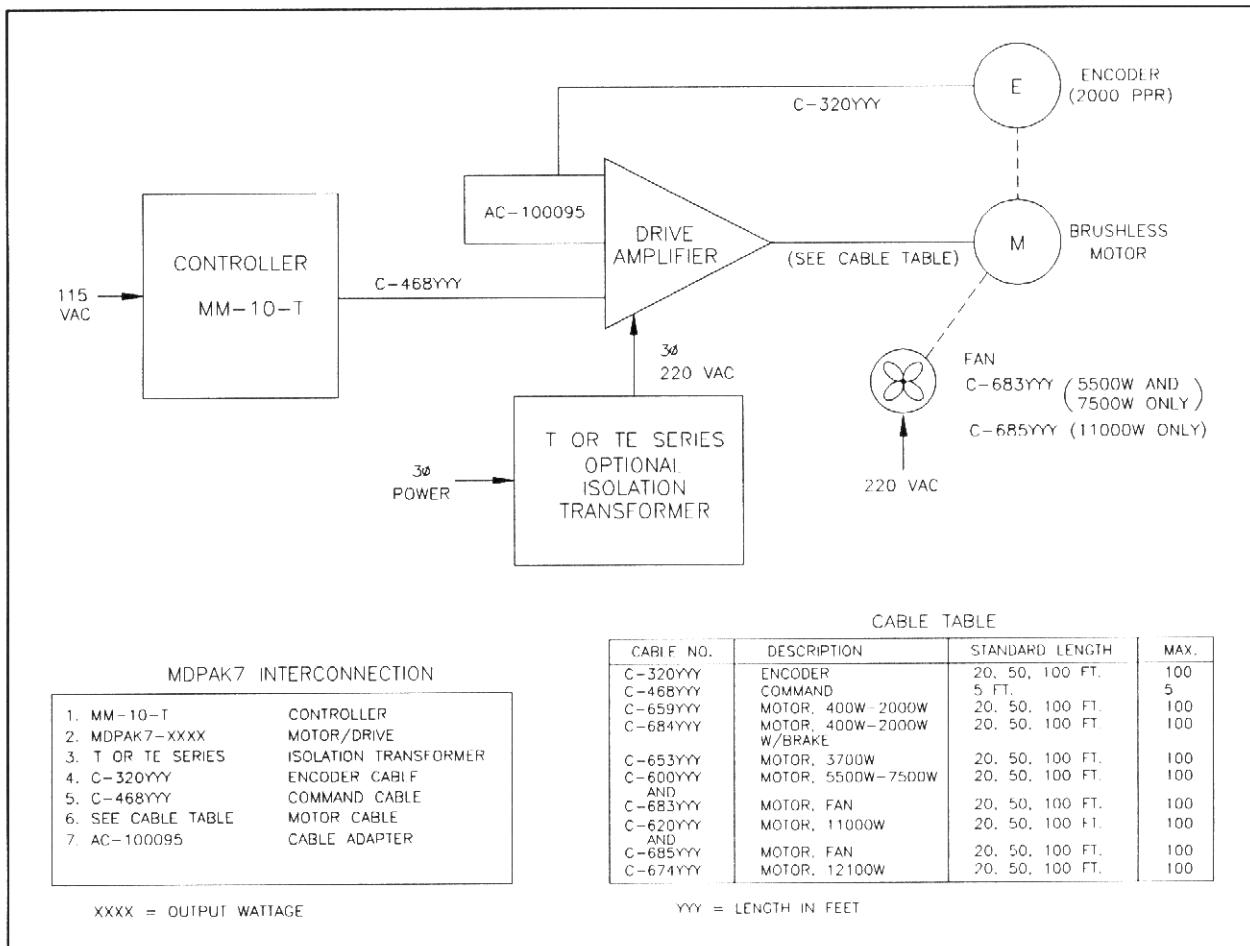
Figure 2.2 - MDPAK7 Connection To Single Axis Positioner
