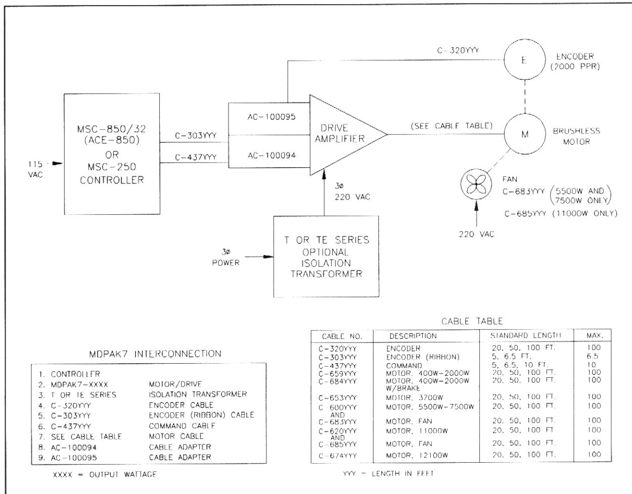
**Figure 2.1 - MDPAK7 Connection To Multi-Axis Positioner**
