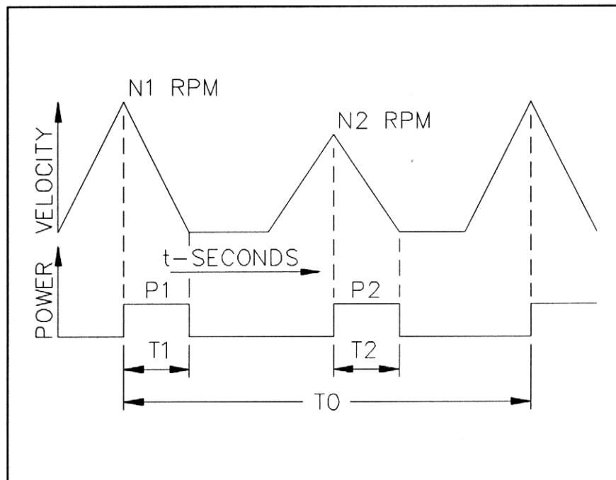
Figure 5.10 - External Regenerative Resistor
