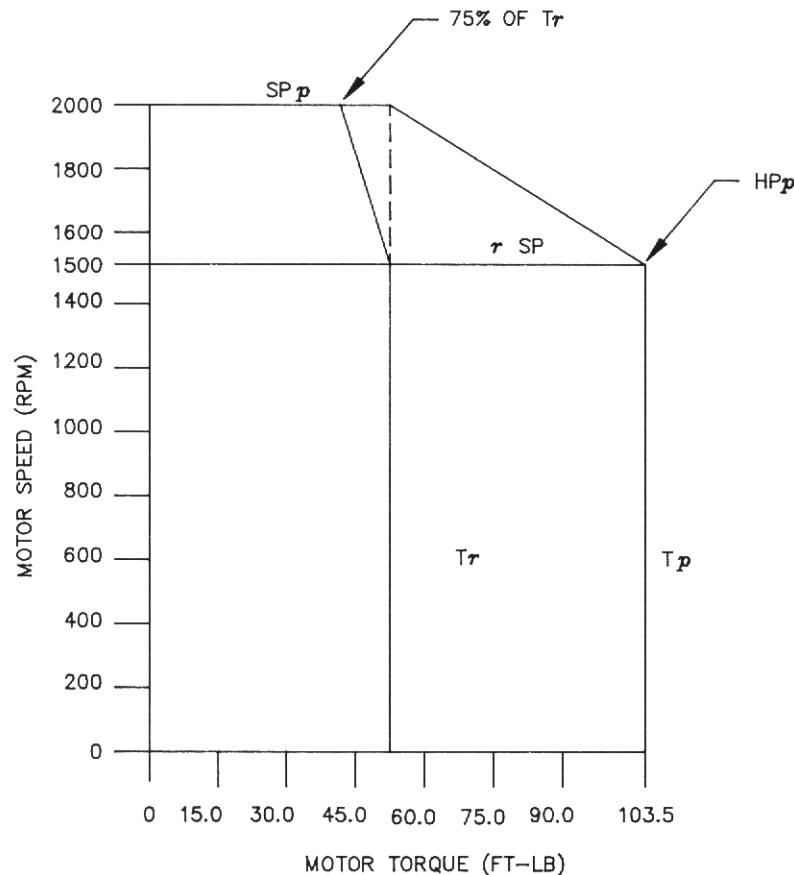
SPEED TEST POINT SCALING: SPEED (RPM) = OUTPUT VOLTS \* SSCL (PARAMETER SSCL DEFAULTS TO 2000 RPM)
