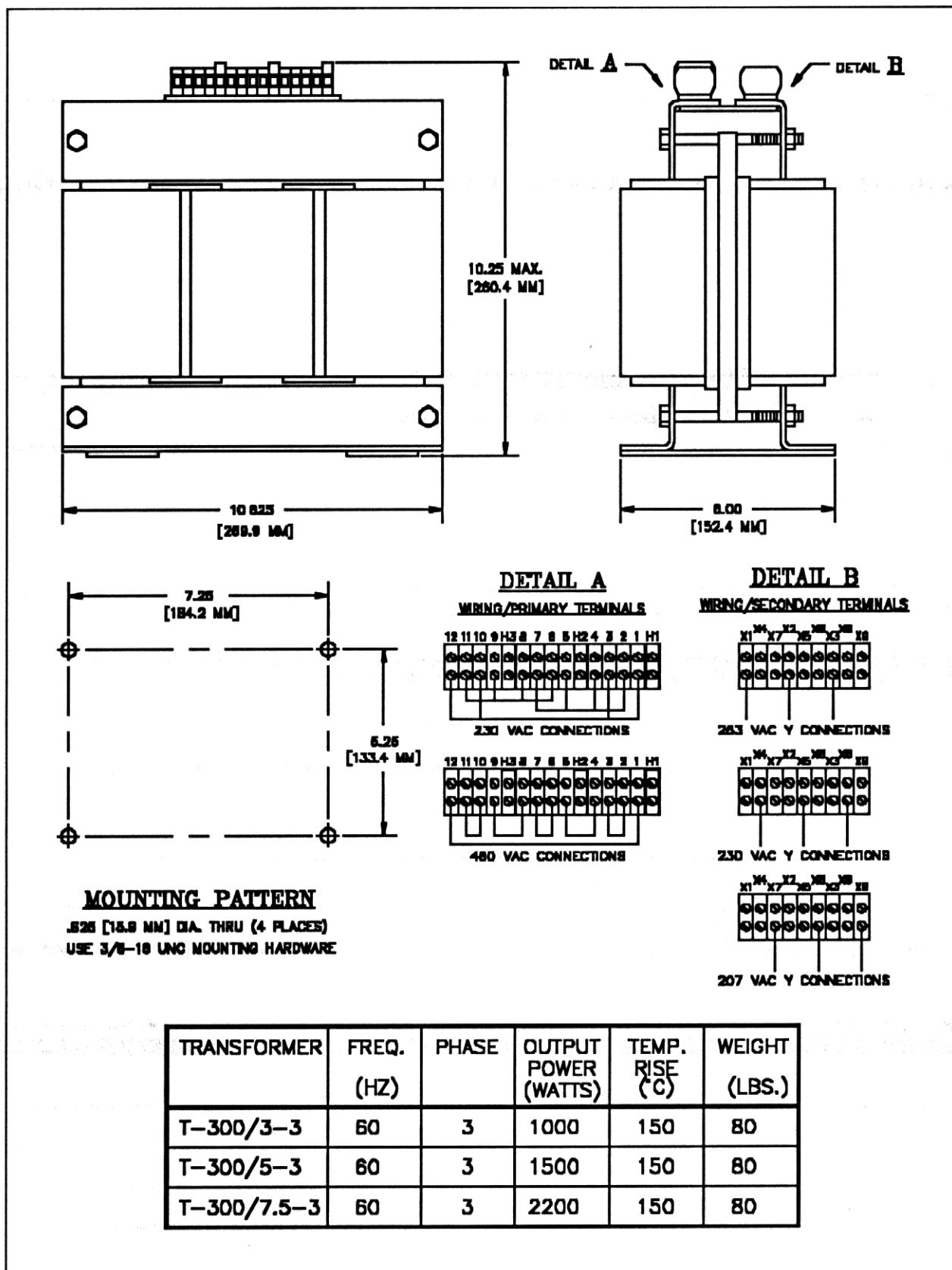
Figure 5.13 - Panel-Mount Transformer Dimensions and Connections
