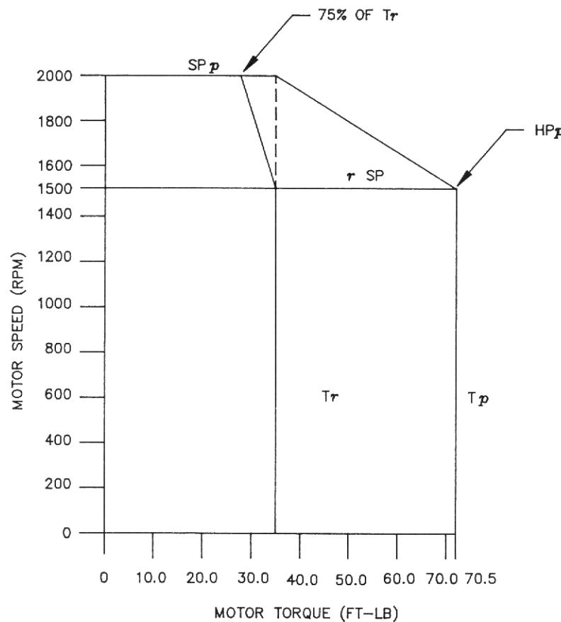
SPEED TEST POINT SCALING: SPEED (RPM) = OUTPUT VOLTS \* SSCL ( PARAMETER SSCL
