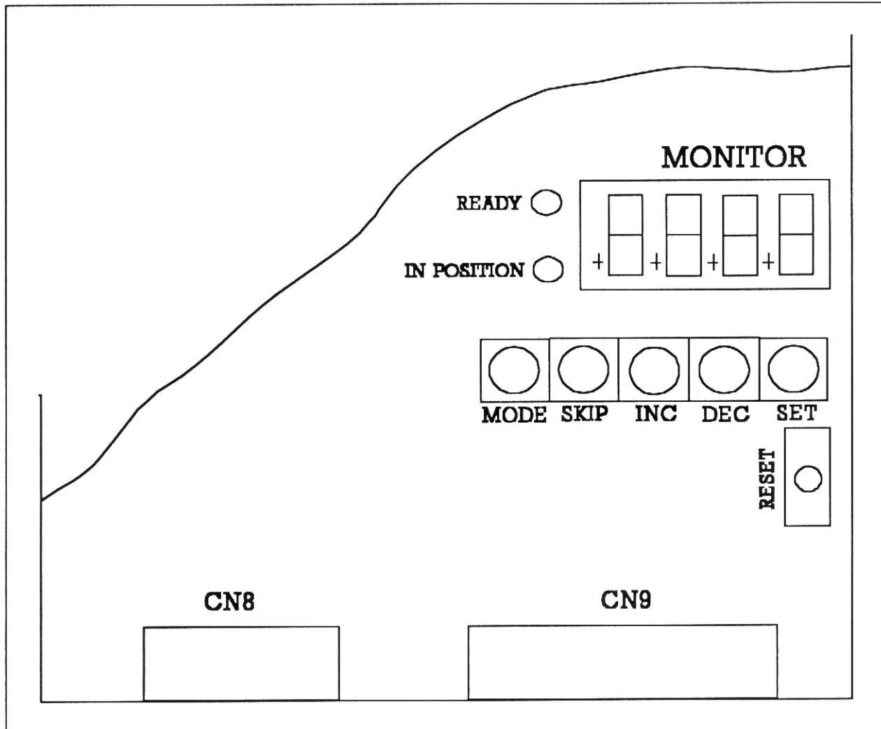
Figure 4.1 - Servo Drive Monitor & Pushbuttons
