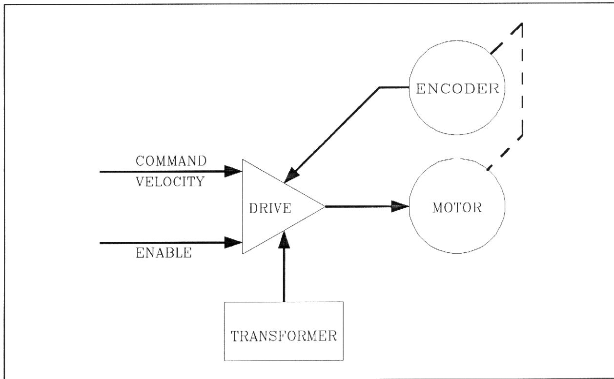
Figure 1.3 - Velocity Loop
