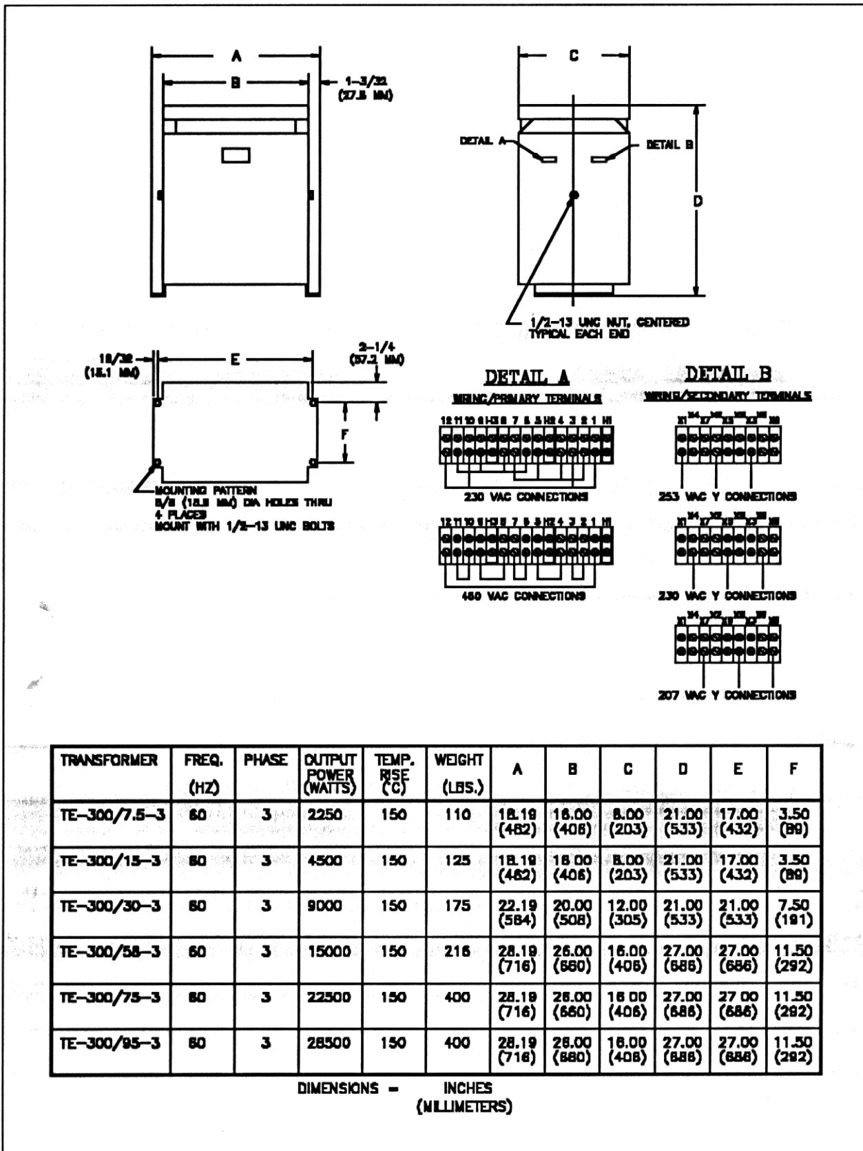
Figure 5.14 - Free-Standing Transformer Dimensions and Connections
