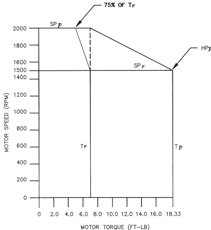
SPEED TEST POINT SCALING: SPEED (RPM) =  $\frac{\text{OUTPUT VOLTS} * \text{SSCL}}{10}$  (PARAMETER SSCL DEFAULTS TO 2000 RPM)
