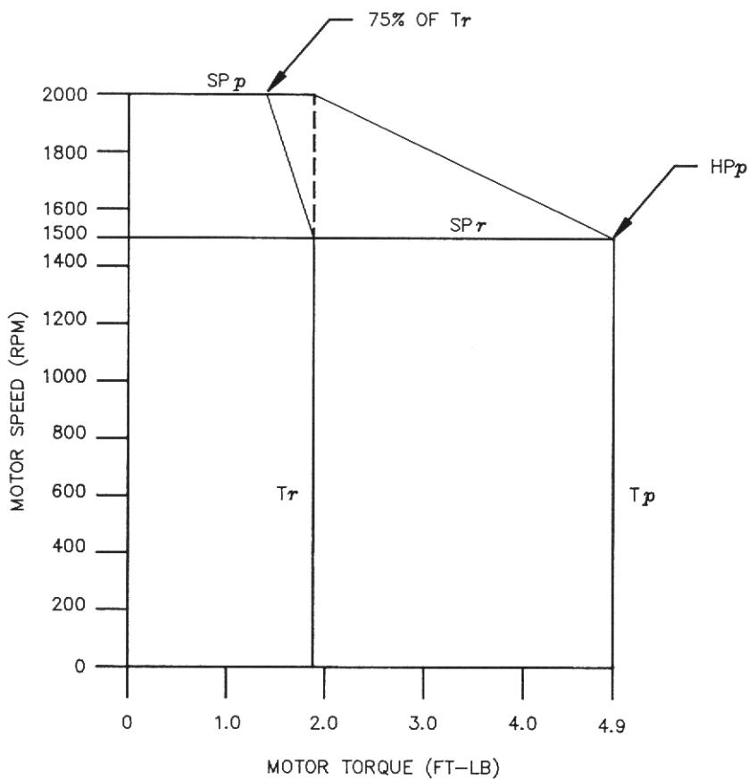
SPEED TEST POINT SCALING: SPEED (RPM) =  $\frac{\text{OUTPUT VOLTS} * \text{SSCL}}{10}$  (PARAMETER SSCL DEFAULTS TO 2000 RPM)
