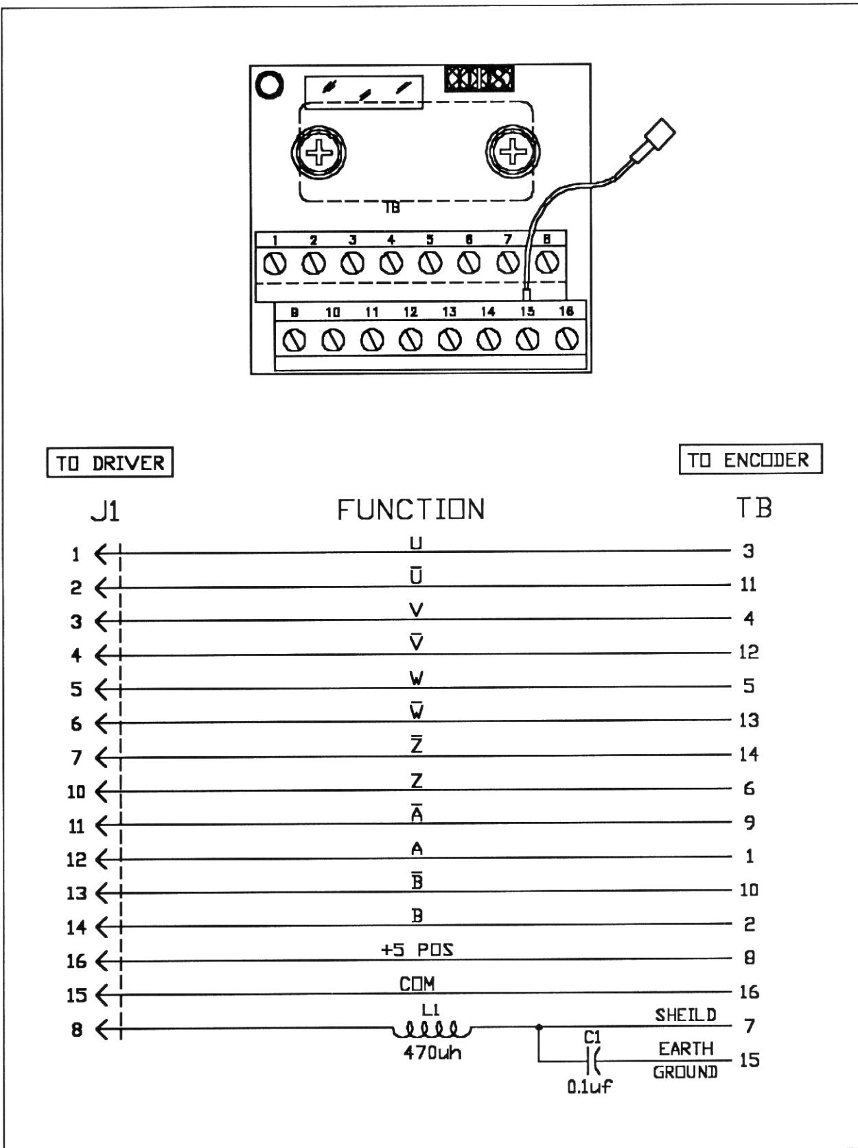
Figure 5.8 - AC-100095 Cable Adaptor
