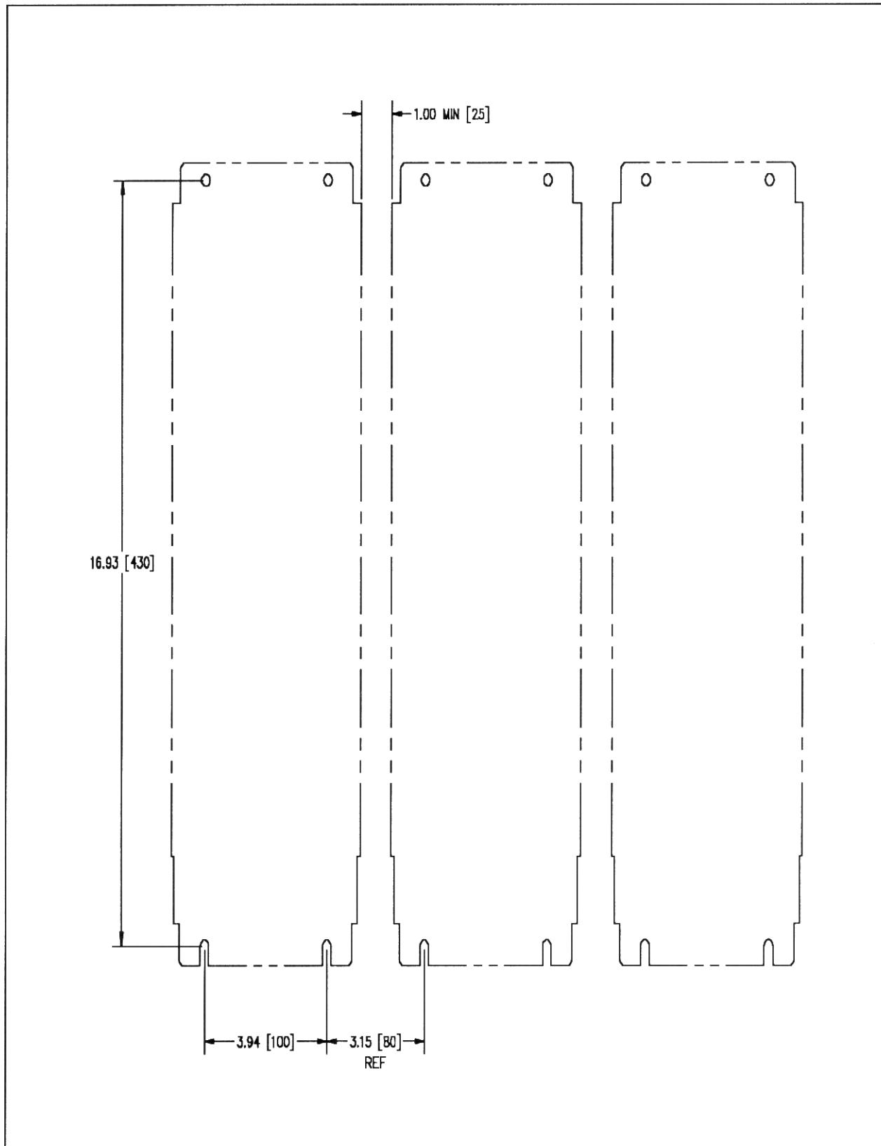
Figure 3.3 - BSD7-R0400 Thru BSD7-R3700 Drivers Mounting Plate
