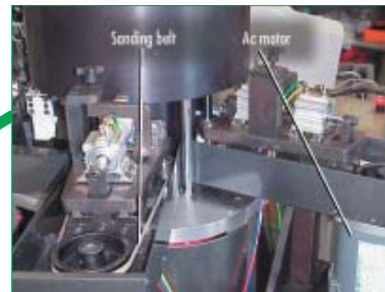
A pair of belt sanders removes runner residue left behind by the lathe. Either one or both of the sanders are used, depending on ball design.
