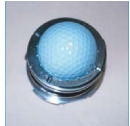
An as-molded ball sitting in the mold lower half shows the small (0.040-in. tall) protrusions about its equator. The protrusions are purposely put there for alignment in ball polishing machines.
