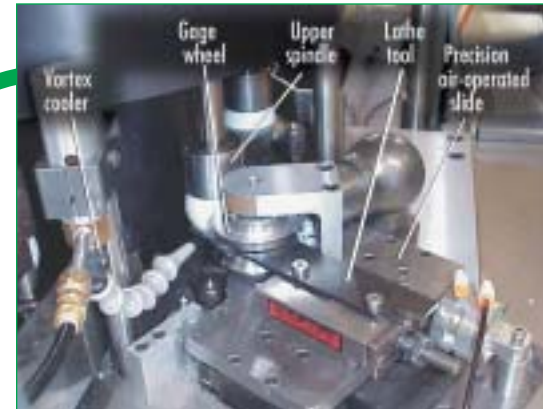
A ball spins between an upper and lower spindle as a precision, air-operated slide moves the lathe tool (cuts off runners) to a depth controlled by the gage wheels. A vortex cooler delivers chilled air to the area and clears away debris.
