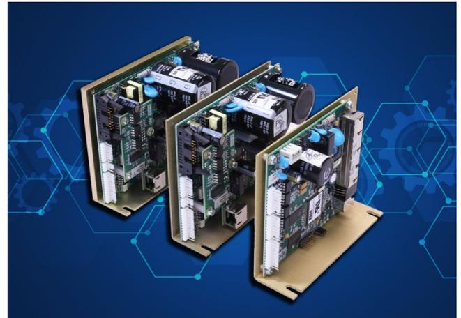
The digital drive interface option bypasses the normal analog circuit path to allow access to the digital registers which control the operation of the speed control loop. Using the universal RS-485 device bus with Modbus RTU as its connectivity scheme, the digital drive is reachable from a variety of HMI, PLC and PC type controllers. The RS485 multi-drive configuration permits drive networks of up to 16 units.
