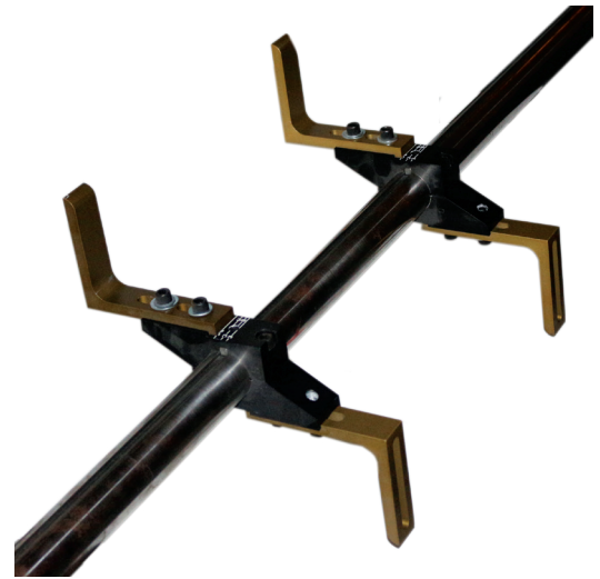
Figure 2 Picture showing one finger set on one axis of a typical machine. Fingers are adjustable along the axis. The servomotor that drives this axis is not shown.
