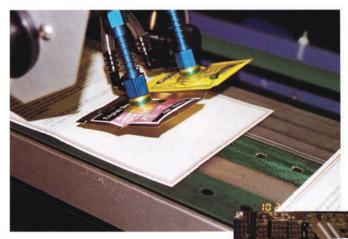
The Pack-Smart 911RD Rotary Placer Machine uses an Industrial Indexing System DeltaMax 1½-axis servosystem to control rotational speed of the arms. The arms carry suction cups to pick up oddly shaped objects. The servosystem also monitors envelope placement on the conveyor belt.
