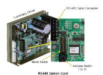
operation of the speed control loop. Using the universal Rs485 device bus with Modbus RTU as its connectivity scheme, the digital drive is reachable from a variety of HMI, PLC and PC type controllers. The Rs485 multi-drive configuration permits drive networks of up to 16 units.
