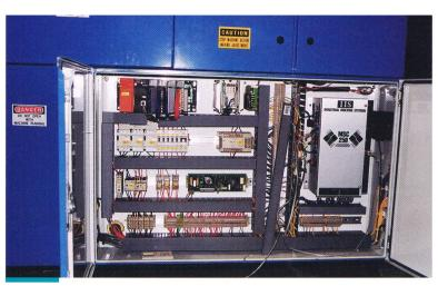
A new servocontrolled sheeter built by VITS America, Blauvelt, N.Y., operates under an **Industrial Indexing Systems** MSC-250,  $2^1/_2$  axis servocontroller. Two Delta Drivers deliver the motion commands to two 5.6-kW precision servomotors that power the infeed rollers and cutting cylinder. Setup of the VITS sheeter is fast and simple, thanks to menu-driven operation and easy-to-use controls.
